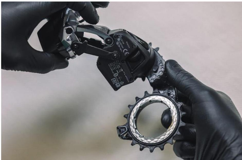
Before you mount the derailleur back to the bike, make sure the movement of the cage is smooth. Note that SRAM AXS derailleurs have a hydraulic clutch therefore you will notice its resistance.
