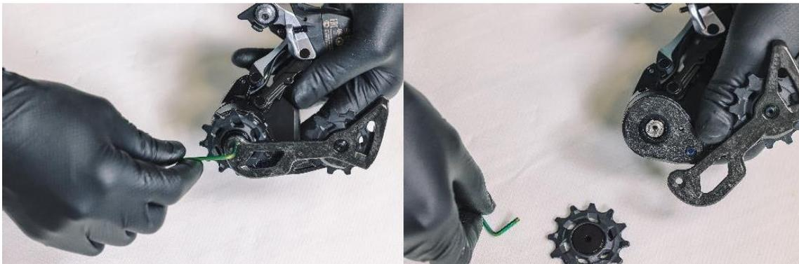
Using a 2.5 mm allen key to unscrew the bolt holding the upper pulley wheel. This will allow you to rotate the cage plate and gain access to the special locking nut holding the cage to the derailleur.
