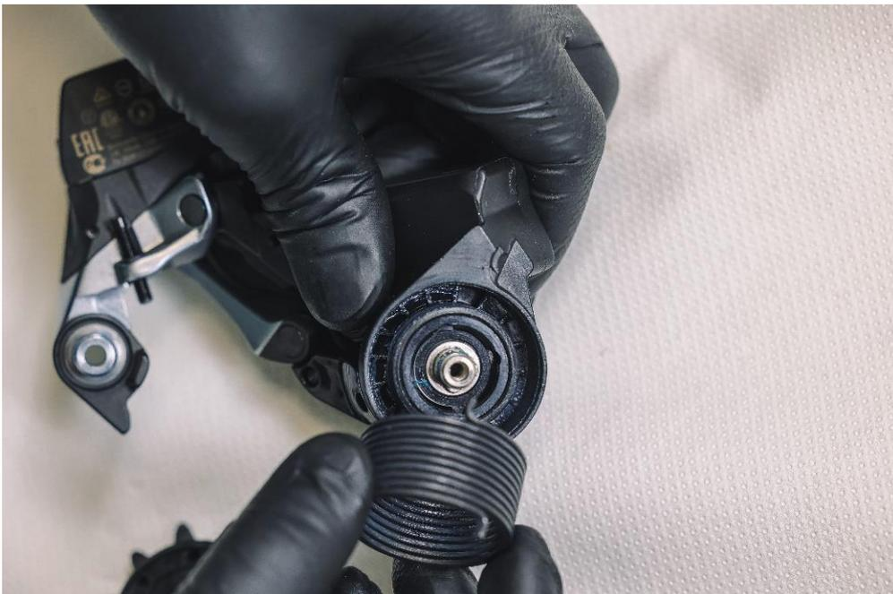
Insert one end of the spring into the recess that is slightly deeper than the rest. The spring is symmetric so it is not important which end of the spring you insert.
