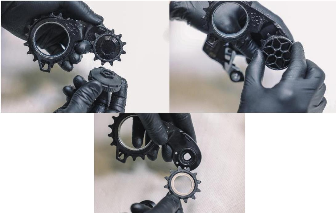
Use provided locking tool to open the locking holding upper pulley wheel.
