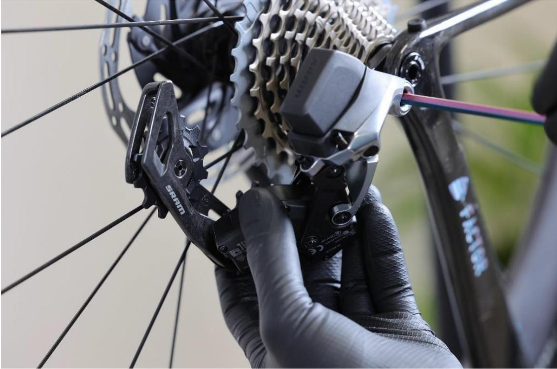
Using a 5 mm Allen key, unscrew the main mounting bolt and remove the derailleur
